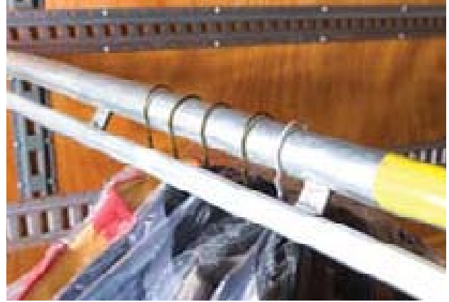
Bar rotates to lock garments in place.
